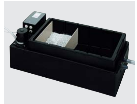
Fig. 39: Granulate neutralisation with condensate lifting pump – applicable for condensate volumes up to 210 l/h, which equals approx. 1500 kW output
