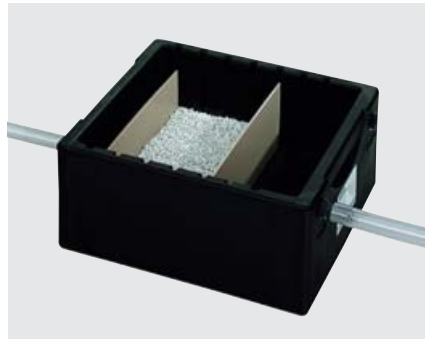
Fig. 38: Granulate neutralisation for condensate volumes from gas fired combustion equipment up to 70 l/h, which equals approx. 500 kW output
