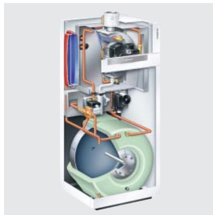
Fig. 45: Vitodens 333 – compact gas fired condensing boiler, 4.5 to 26.0 kW with integral loading cylinder (86 litres capacity)
